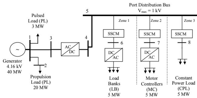
Fig. 2. The Navy Ship Reduced IPS Model
