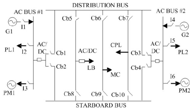
Fig. 1. The Navy Ship Integrated Power System (IPS) Model
