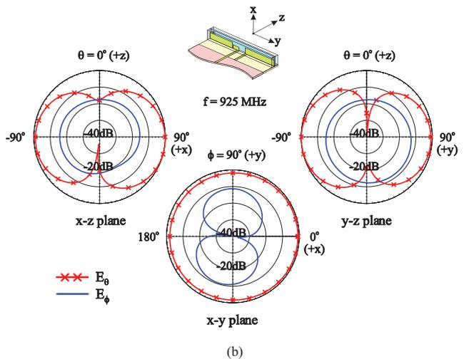
**Figure 7** Measured radiation pattern for the proposed antenna. (a) 859 MHz; (b) 925 MHz. [Color figure can be viewed in the online issue, which is available at [www.interscience.wiley.com](http://www.interscience.wiley.com)]
