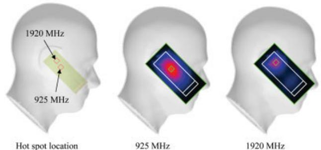
**Figure 12** Simulated SAR distributions for the proposed antenna at 925 and 1920 MHz. (a) Antenna at the top position. (b) Antenna at the bottom position. [Color figure can be viewed in the online issue, which is available at [www.interscience.wiley.com](http://www.interscience.wiley.com)]
