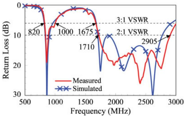
**Figure 2** Measured and simulated return loss for the proposed antenna. [Color figure can be viewed in the online issue, which is available at [www.interscience.wiley.com](http://www.interscience.wiley.com)]
