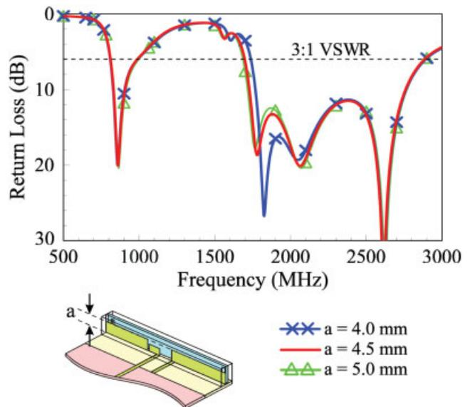
**Figure 4** Simulated return loss as a function of the width  $a$  of the radiating portion in layer 1 of the proposed antenna. [Color figure can be viewed in the online issue, which is available at [www.interscience.wiley.com](http://www.interscience.wiley.com)]
