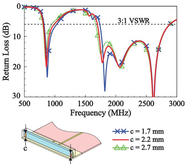
**Figure 6** Simulated return loss as a function of the length  $c$  of the tuning slits in layer 2 of the proposed antenna. [Color figure can be viewed in the online issue, which is available at [www.interscience.wiley.com](http://www.interscience.wiley.com)]
