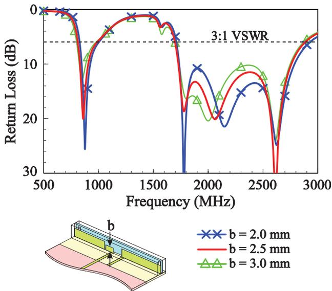
**Figure 5** Simulated return loss as a function of the width  $b$  of the coupling pad in layer 1 of the proposed antenna. [Color figure can be viewed in the online issue, which is available at [www.interscience.wiley.com](http://www.interscience.wiley.com)]
