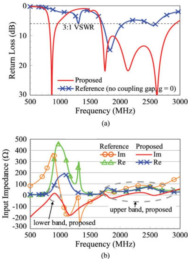
**Figure 3** Simulated (a) return loss and (b) input impedance of the proposed and reference antennas. [Color figure can be viewed in the online issue, which is available at [www.interscience.wiley.com](http://www.interscience.wiley.com)]
