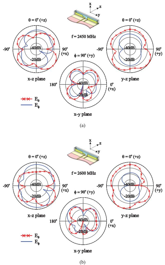
**Figure 9** Measured radiation pattern for the proposed antenna. (a) 2450 MHz. (b) 2600 MHz. [Color figure can be viewed in the online issue, which is available at [www.interscience.wiley.com](http://www.interscience.wiley.com)]
