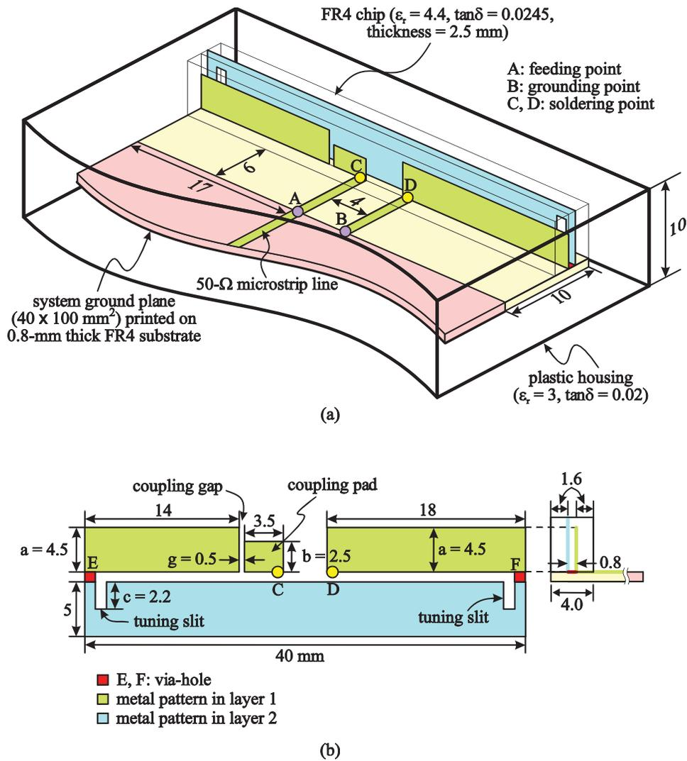
**Figure 1** (a) Geometry of the seven-band folded-loop chip antenna for WWAN/WLAN/WiMAX operation in the mobile phone; the antenna is enclosed by a 1-mm thick plastic housing. (b) Dimensions of the metal pattern inside the chip antenna in its unfolded structure. [Color figure can be viewed in the online issue, which is available at [www.interscience.wiley.com](http://www.interscience.wiley.com)]
