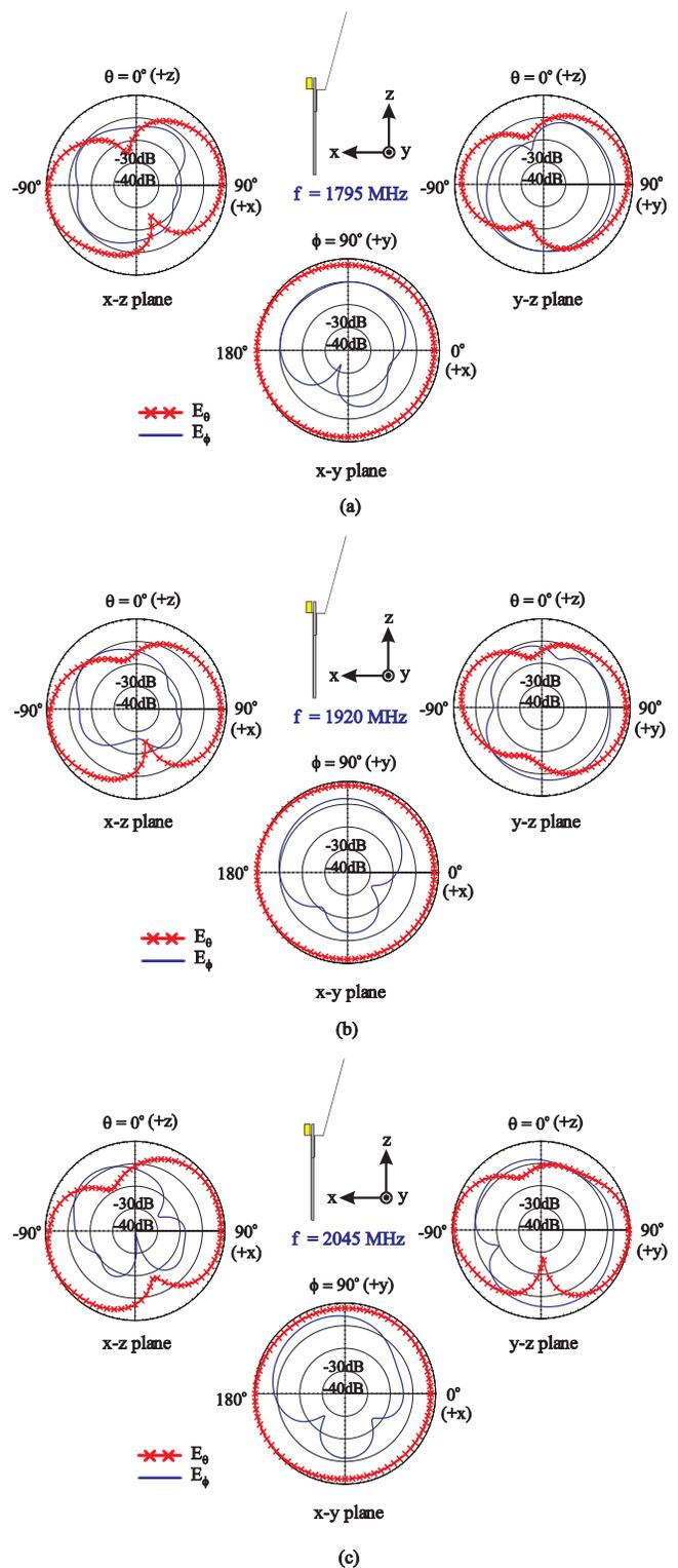
**Figure 8** Measured radiation patterns at (a) 1795 MHz, (b) 1920 MHz, and (c) 2045 MHz for the proposed PIFA. [Color figure can be viewed in the online issue, which is available at [www.interscience.wiley.com](http://www.interscience.wiley.com)]
