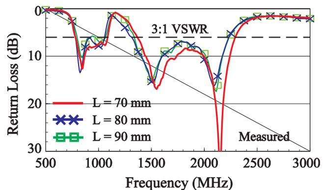
**Figure 6** Measured return loss for the proposed PIFA as a function of the length  $L$  of the main ground and upper ground; other parameters are the same as given in Figure 1. [Color figure can be viewed in the online issue, which is available at [www.interscience.wiley.com](http://www.interscience.wiley.com)]
