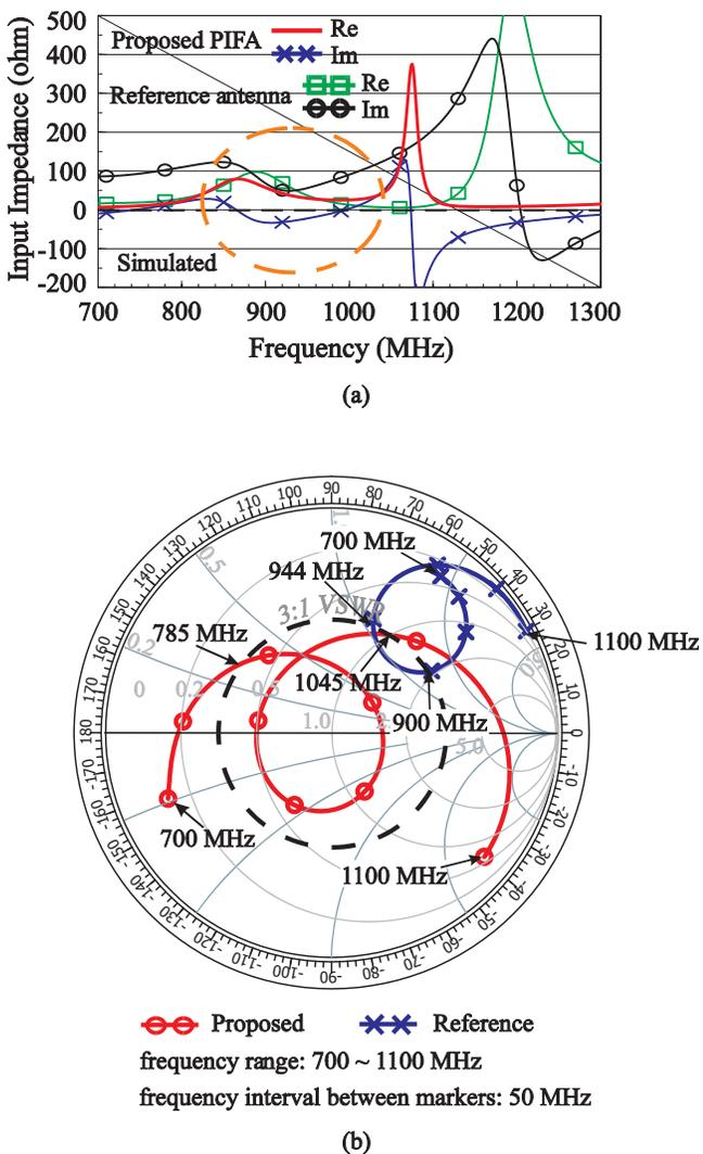
**Figure 4** (a) Simulated input impedance versus frequency and (b) simulated input impedance on the Smith chart for the reference antenna studied in Figure 3 and the proposed PIFA. Only the results for the lower band of the antenna are shown. [Color figure can be viewed in the online issue, which is available at [www.interscience.wiley.com](http://www.interscience.wiley.com)]
