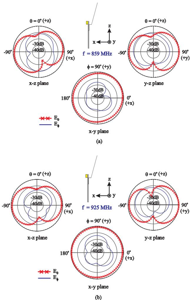
**Figure 7** Measured radiation patterns at (a) 859 MHz and (b) 925 MHz for the proposed PIFA. [Color figure can be viewed in the online issue, which is available at [www.interscience.wiley.com](http://www.interscience.wiley.com)]
