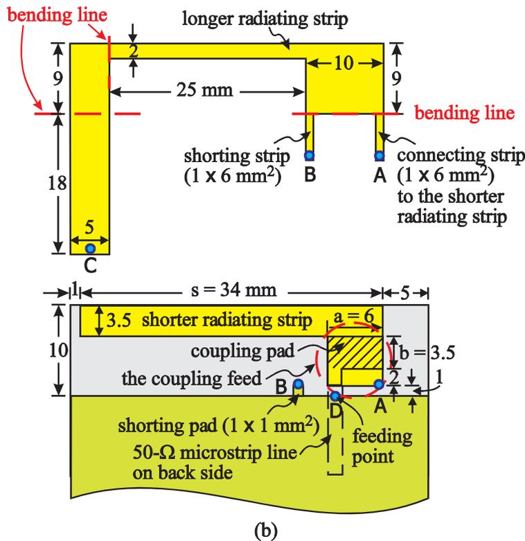
**Figure 1** (a) Geometry of the proposed PIFA for the penta-band folder-type mobile phone. (b) Dimensions of the proposed PIFA. [Color figure can be viewed in the online issue, which is available at [www.interscience.wiley.com](http://www.interscience.wiley.com)]
