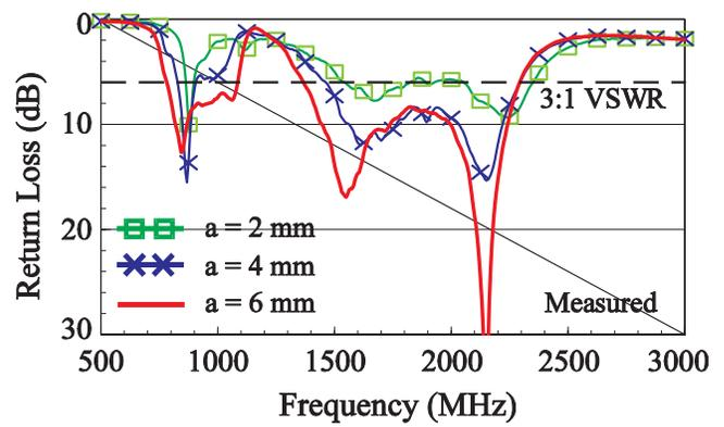
**Figure 5** Measured return loss for the proposed PIFA as a function of the length  $a$  of the coupling pad; other parameters are the same as given in Figure 1. [Color figure can be viewed in the online issue, which is available at [www.interscience.wiley.com](http://www.interscience.wiley.com)]
