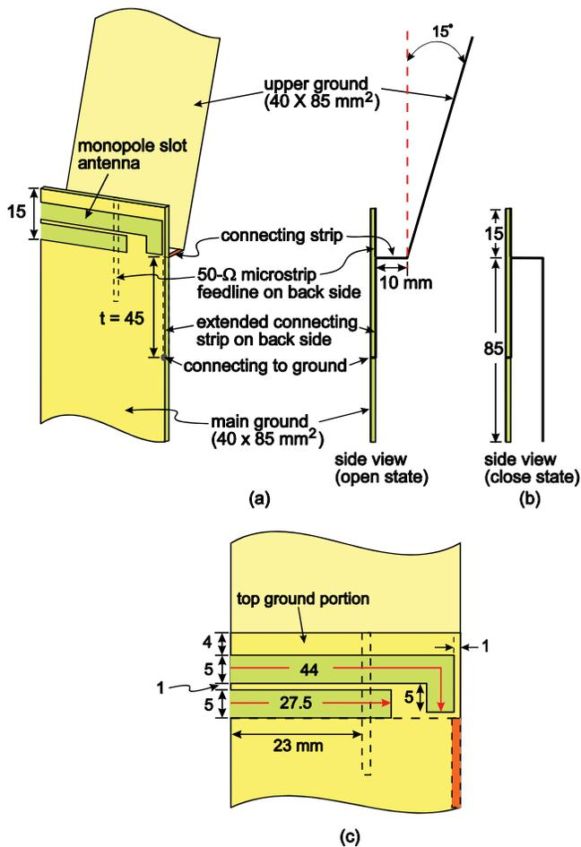
**Figure 1** (a) Configuration of the penta-band monopole slot antenna for folder-type mobile phone in the open state (talk condition). (b) Side view of the mobile phone in the close state (standby condition). (c) Dimensions of the antenna. [Color figure can be viewed in the online issue, which is available at [www.interscience.wiley.com](http://www.interscience.wiley.com)]
