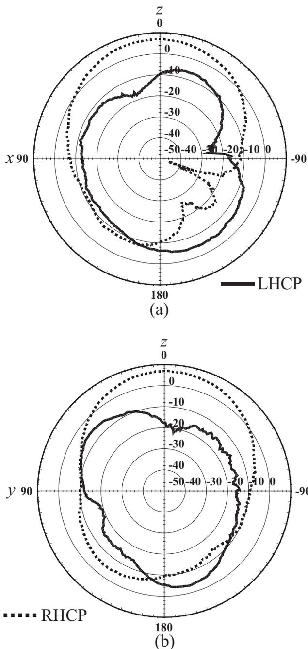
**Figure 6** Radiation patterns of the RHCP mode of Prototype A measured at 3000 MHz. (a)  $x$ - $z$  plane (b)  $y$ - $z$  plane
