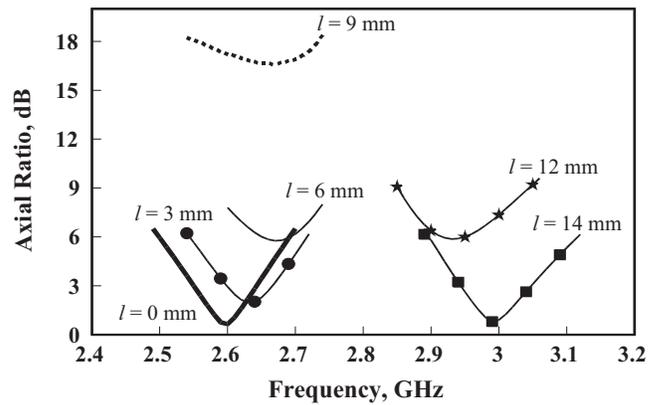
**Figure 2** Simulated results for the effects of various  $l$  on the axial ratio
