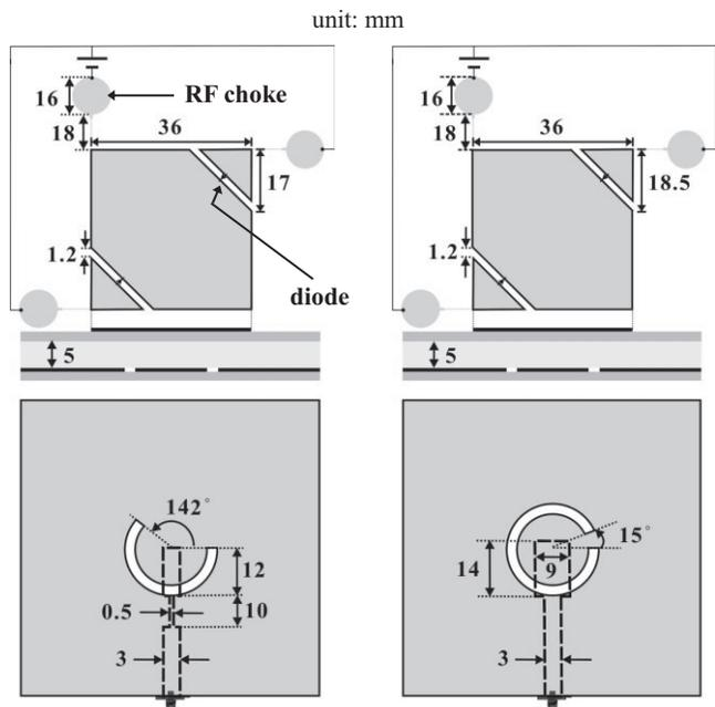
**Figure 3** Designs of the two constructed prototypes
