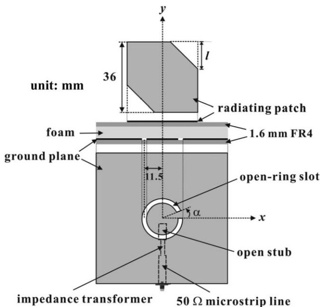
**Figure 1** Geometry of the proposed reconfigurable microstrip antenna
