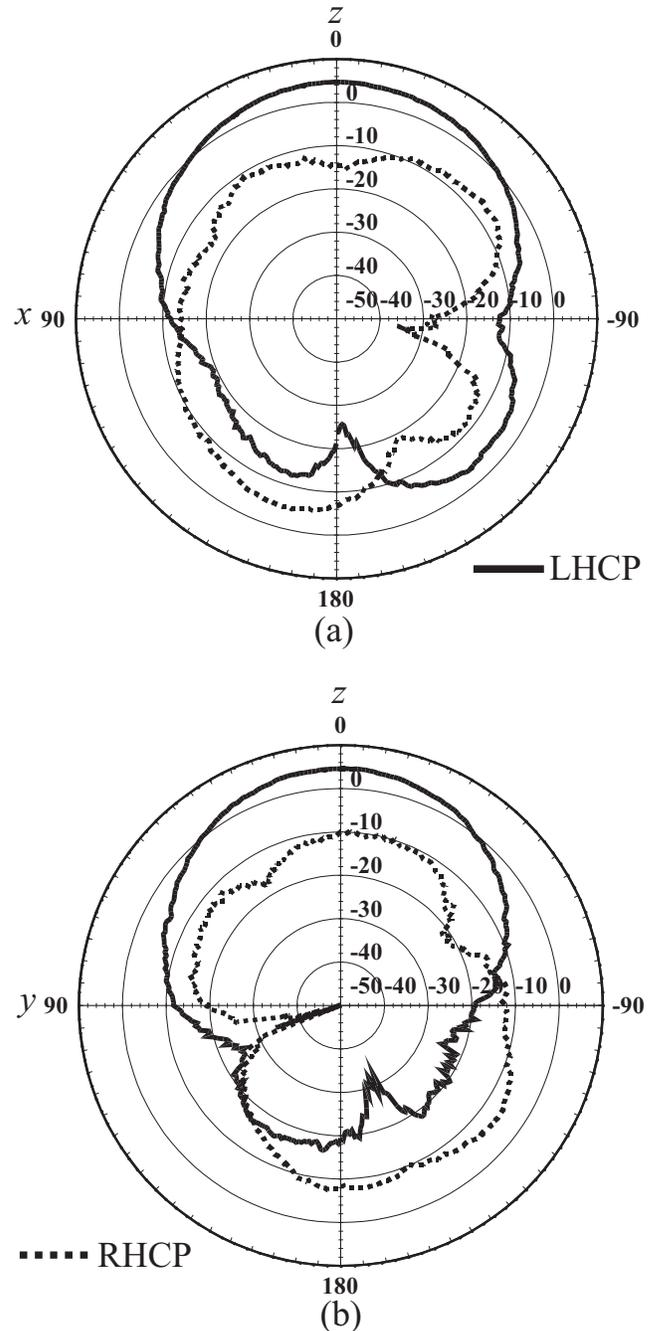
**Figure 5** Radiation patterns of the LHCP mode of Prototype A measured at 2430 MHz. (a)  $x$ - $z$  plane (b)  $y$ - $z$  plane
