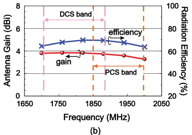
**Figure 9** Measured antenna gain and simulated radiation efficiency for the hybrid antenna. (a) The GSM850/900 bands. (b) The DCS/PCS bands. [Color figure can be viewed in the online issue, which is available at [www.interscience.wiley.com](http://www.interscience.wiley.com)]
