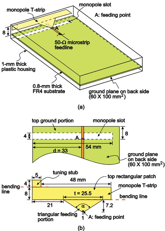
**Figure 1** (a) Configuration of the proposed internal multiband hybrid antenna enclosed by a 1-mm thick plastic mobile phone housing. (b) Dimensions of the monopole slot and monopole T-strip of the hybrid antenna. [Color figure can be viewed in the online issue, which is available at [www.interscience.wiley.com](http://www.interscience.wiley.com)]
