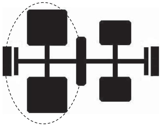
**Figure 1** Geometry of a third-order bandpass filter consisted of ACMR
