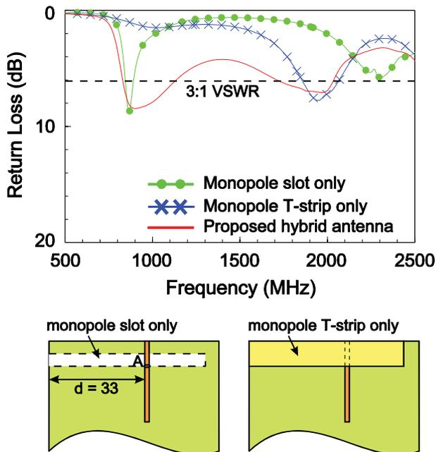
**Figure 3** Comparison of the simulated return loss for the proposed hybrid antenna, the case with the monopole slot only, and the case with the monopole T-strip only. [Color figure can be viewed in the online issue, which is available at [www.interscience.wiley.com](http://www.interscience.wiley.com)]
