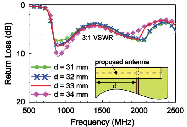
**Figure 4** Simulated return loss as a function of the feedline location  $d$ ; other dimensions are the same as in Figure 1. [Color figure can be viewed in the online issue, which is available at [www.interscience.wiley.com](http://www.interscience.wiley.com)]
