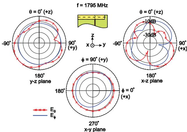
**Figure 7** Measured radiation patterns at 1795 MHz for the hybrid antenna. [Color figure can be viewed in the online issue, which is available at [www.interscience.wiley.com](http://www.interscience.wiley.com)]
