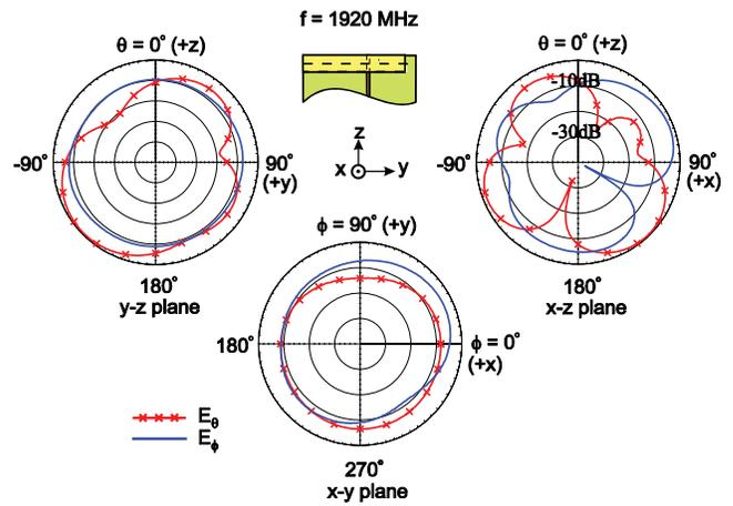
**Figure 8** Measured radiation patterns at 1920 MHz for the hybrid antenna. [Color figure can be viewed in the online issue, which is available at [www.interscience.wiley.com](http://www.interscience.wiley.com)]
