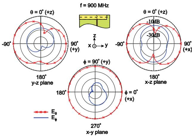
**Figure 6** Measured radiation patterns at 900 MHz for the hybrid antenna. [Color figure can be viewed in the online issue, which is available at [www.interscience.wiley.com](http://www.interscience.wiley.com)]
