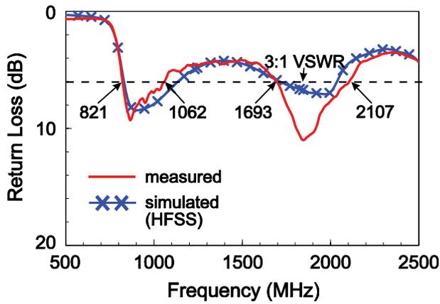
**Figure 2** Measured and simulated return loss for the proposed hybrid antenna. [Color figure can be viewed in the online issue, which is available at [www.interscience.wiley.com](http://www.interscience.wiley.com)]
