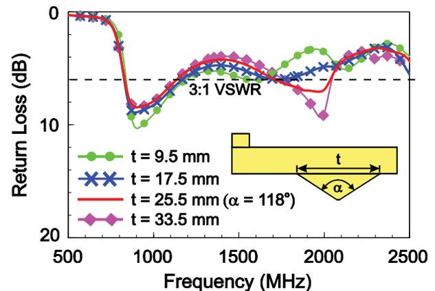
**Figure 5** Simulated return loss as a function of the length  $t$  of the triangular feeding portion; other dimensions are the same as in Figure 1. [Color figure can be viewed in the online issue, which is available at [www.interscience.wiley.com](http://www.interscience.wiley.com)]
