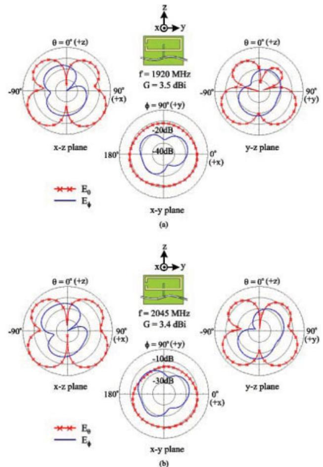
**Figure 8** Measured radiation patterns for the antenna studied in Figure 2: (a) 1920 MHz; (b) 2045 MHz. [Color figure can be viewed in the online issue, which is available at [www.interscience.wiley.com](http://www.interscience.wiley.com)]
