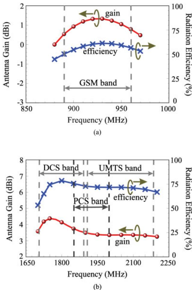
**Figure 9** Measured antenna gain and simulated (HFSS) radiation efficiency for the antenna studied in Figure 2: (a) The lower band; (b) The upper band. [Color figure can be viewed in the online issue, which is available at [www.interscience.wiley.com](http://www.interscience.wiley.com)]
