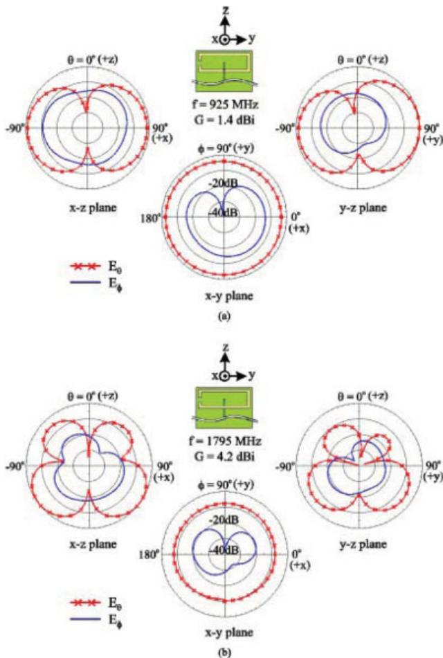
**Figure 7** Measured radiation patterns for the antenna studied in Figure 2: (a) 925 MHz; (b) 1795 MHz. [Color figure can be viewed in the online issue, which is available at [www.interscience.wiley.com](http://www.interscience.wiley.com)]
