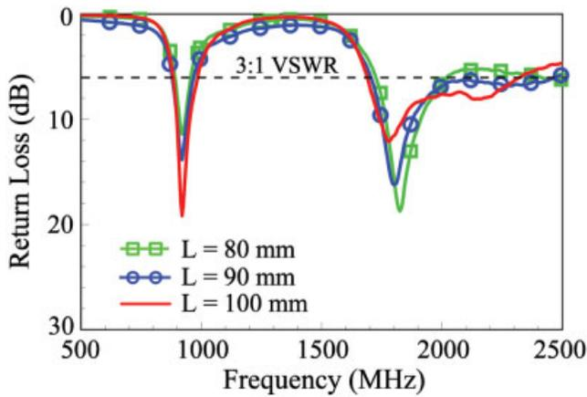
**Figure 4** Measured return loss as a function of ground-plane length  $L$ . Other dimensions are the same as studied in Figure 2. [Color figure can be viewed in the online issue, which is available at [www.interscience.wiley.com](http://www.interscience.wiley.com)]
