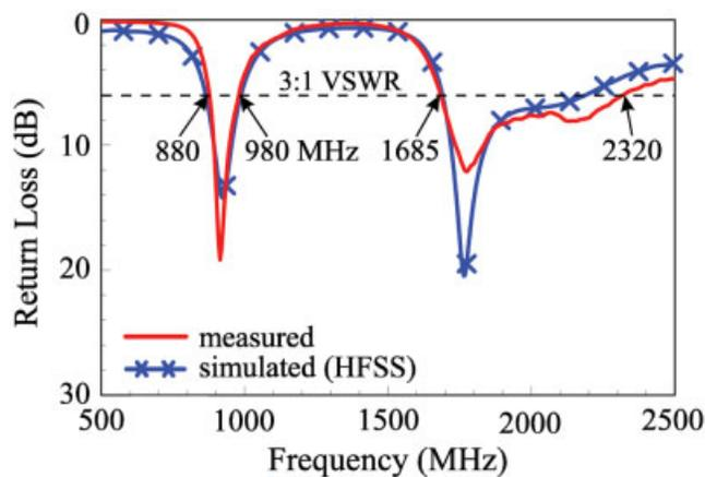
**Figure 2** Measured and simulated (HFSS) return loss for the proposed antenna. [Color figure can be viewed in the online issue, which is available at [www.interscience.wiley.com](http://www.interscience.wiley.com)]
