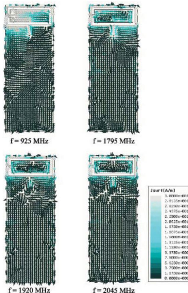
**Figure 3** Simulated (HFSS) excited surface currents at 925, 1795, 1920, and 2045 MHz in the system ground plane of the mobile phone studied in Figure 2. [Color figure can be viewed in the online issue, which is available at [www.interscience.wiley.com](http://www.interscience.wiley.com)]
