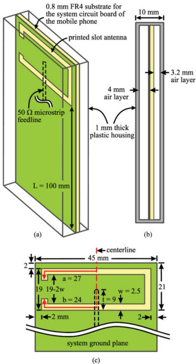
**Figure 1** (a) Geometry of the proposed folded slot antenna printed on the system circuit board of the mobile phone; (b) Side view of the studied mobile phone with a plastic housing; (c) Detailed dimensions of the antenna. [Color figure can be viewed in the online issue, which is available at [www.interscience.wiley.com](http://www.interscience.wiley.com)]
