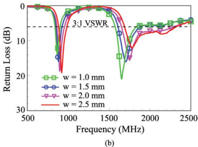
**Figure 5** Measured return loss (a) as a function of tuning-stub length  $t$  and (b) as a function of slot width  $w$ . Other dimensions are the same as studied in Figure 2. [Color figure can be viewed in the online issue, which is available at [www.interscience.wiley.com](http://www.interscience.wiley.com)]
