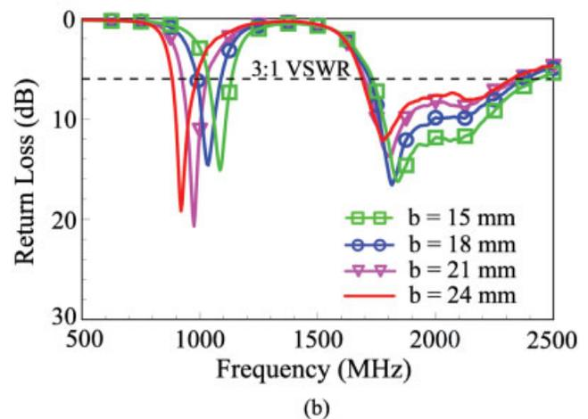
**Figure 6** Measured return loss (a) as a function of end-portion slot length  $a$  and (b) as a function of feed-portion slot length  $b$ . Other dimensions are the same as studied in Figure 2. [Color figure can be viewed in the online issue, which is available at [www.interscience.wiley.com](http://www.interscience.wiley.com)]
