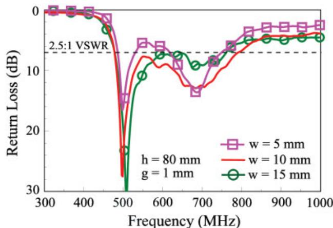
**Figure 6** Measured return loss for the proposed antenna as a function of  $w$  (the width of strip 1); other parameters are the same as studied in Figure 3. [Color figure can be viewed in the online issue, which is available at [www.interscience.wiley.com](http://www.interscience.wiley.com)]
