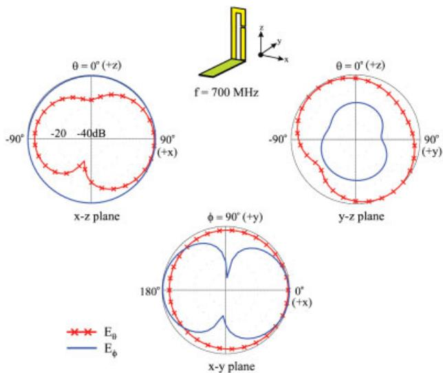
**Figure 8** Simulated radiation patterns at 700 MHz for the proposed antenna studied in Figure 3. [Color figure can be viewed in the online issue, which is available at [www.interscience.wiley.com](http://www.interscience.wiley.com)]
