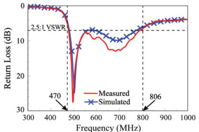
**Figure 3** Measured and simulated return loss for the proposed antenna with  $g = 1$  mm,  $h = 80$  mm, and  $w = 10$  mm. [Color figure can be viewed in the online issue, which is available at [www.interscience.wiley.com](http://www.interscience.wiley.com)]
