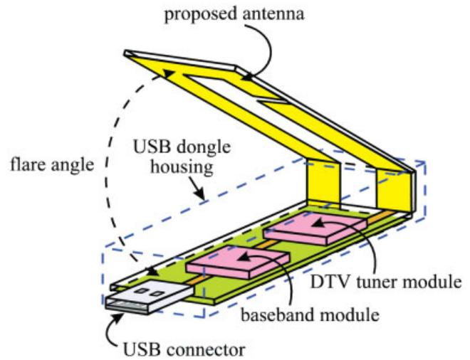
**Figure 2** Example of a promising USB dongle integrated with the proposed antenna. [Color figure can be viewed in the online issue, which is available at [www.interscience.wiley.com](http://www.interscience.wiley.com)]
