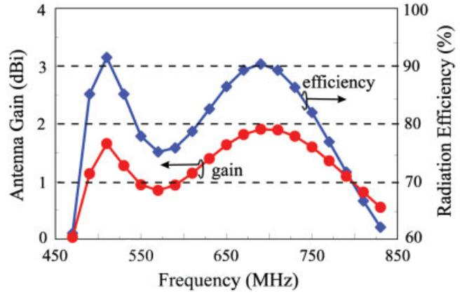
**Figure 9** Simulated antenna gain and radiation efficiency for the proposed antenna studied in Figure 3. [Color figure can be viewed in the online issue, which is available at [www.interscience.wiley.com](http://www.interscience.wiley.com)]
