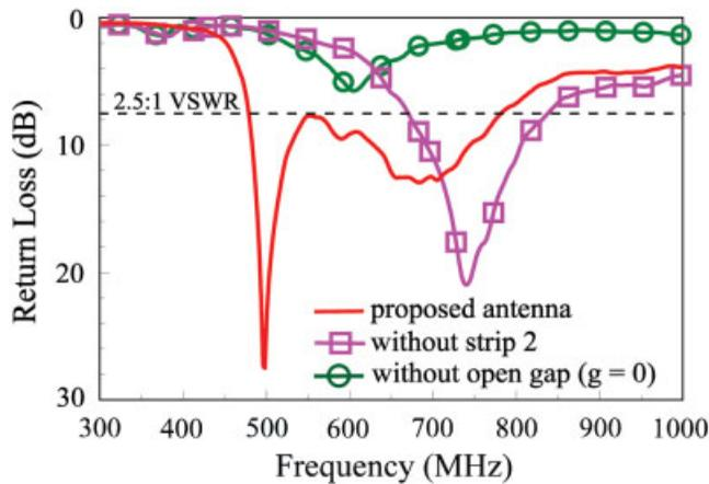
**Figure 4** Measured return loss for the proposed antenna, the antenna without strip 2, and the antenna without the open gap ( $g = 0$ ). The antenna parameters are the same as studied in Figure 3. [Color figure can be viewed in the online issue, which is available at [www.interscience.wiley.com](http://www.interscience.wiley.com)]
