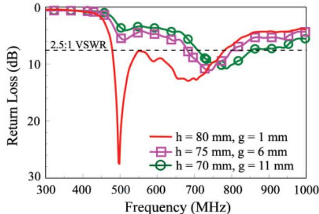
**Figure 5** Measured return loss for the proposed antenna as a function of  $h$  (the length of strip 1) with the total length of  $h$  and  $g$  fixed to be 81 mm; other parameters are the same as studied in Figure 3. [Color figure can be viewed in the online issue, which is available at [www.interscience.wiley.com](http://www.interscience.wiley.com)]
