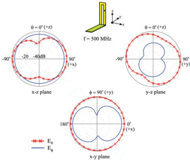
**Figure 7** Simulated radiation patterns at 500 MHz for the proposed antenna studied in Figure 3. [Color figure can be viewed in the online issue, which is available at [www.interscience.wiley.com](http://www.interscience.wiley.com)]
