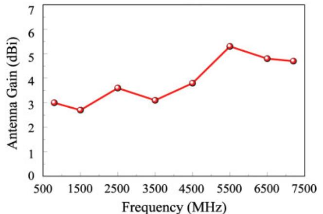
**Figure 10** Measured antenna gain for the proposed antenna studied in Figure 3. [Color figure can be viewed in the online issue, which is available at [www.interscience.wiley.com](http://www.interscience.wiley.com)]
