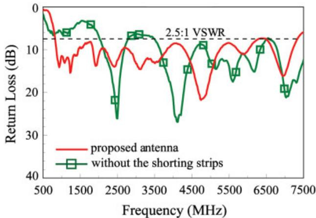
**Figure 4** Measured return loss for the proposed antenna and the case without the shorting strips. [Color figure can be viewed in the online issue, which is available at [www.interscience.wiley.com](http://www.interscience.wiley.com)]
