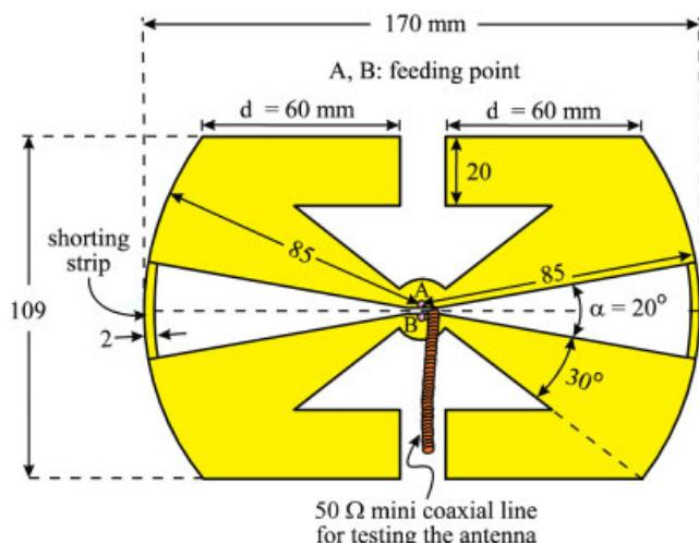
**Figure 1** Geometry of the proposed ultra-wideband planar shorted dipole antenna. [Color figure can be viewed in the online issue, which is available at www.interscience.wiley.com]
