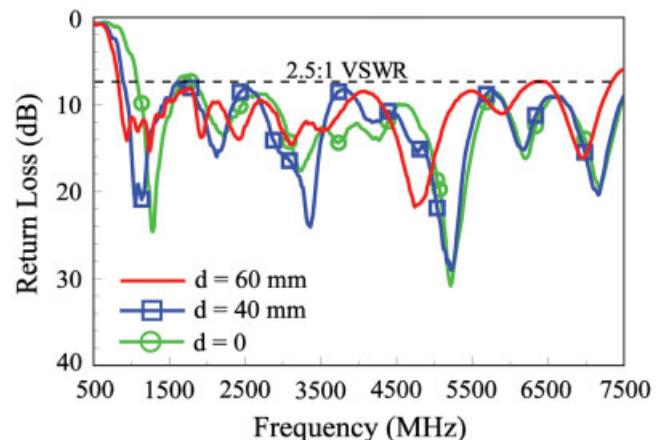
**Figure 6** Measured return loss for the proposed antenna with  $d = 0$ , 40, and 60 mm; other dimensions are the same as given in Figure 1. [Color figure can be viewed in the online issue, which is available at [www.interscience.wiley.com](http://www.interscience.wiley.com)]
