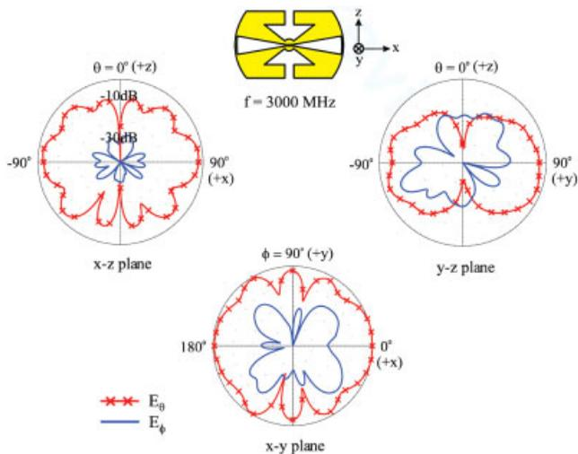
**Figure 8** Measured radiation pattern at 3000 MHz for the proposed antenna studied in Figure 3. [Color figure can be viewed in the online issue, which is available at [www.interscience.wiley.com](http://www.interscience.wiley.com)]
