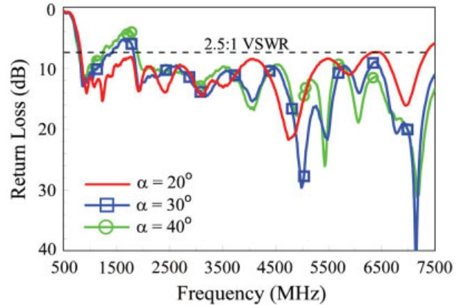
**Figure 5** Measured return loss for the proposed antenna with  $\alpha = 20^\circ$ ,  $30^\circ$ , and  $40^\circ$ ; other dimensions are the same as given in Figure 1. [Color figure can be viewed in the online issue, which is available at [www.interscience.wiley.com](http://www.interscience.wiley.com)]
