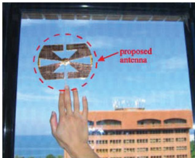
**Figure 2** Photo of the fabricated prototype of the proposed antenna attached on the window pane of the electrical engineering building inside the campus of the National Sun Yat-sen University. [Color figure can be viewed in the online issue, which is available at www.interscience.wiley.com]
