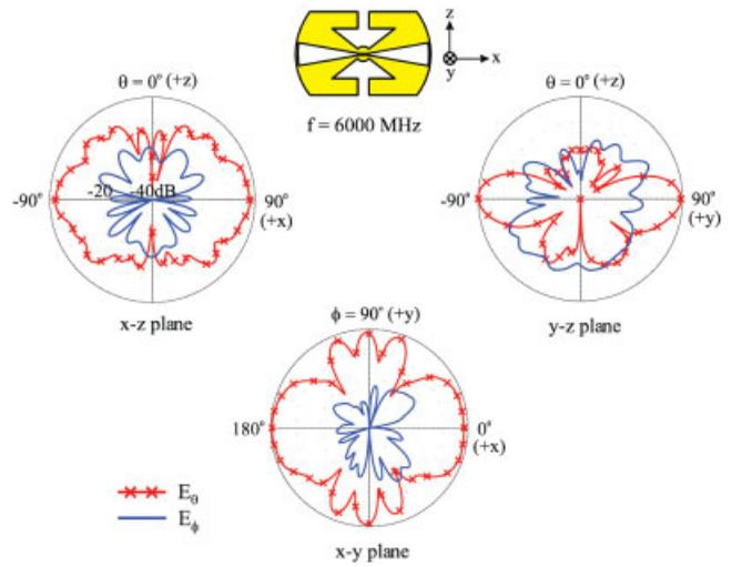
**Figure 9** Measured radiation pattern at 6000 MHz for the proposed antenna studied in Figure 3. [Color figure can be viewed in the online issue, which is available at [www.interscience.wiley.com](http://www.interscience.wiley.com)]
