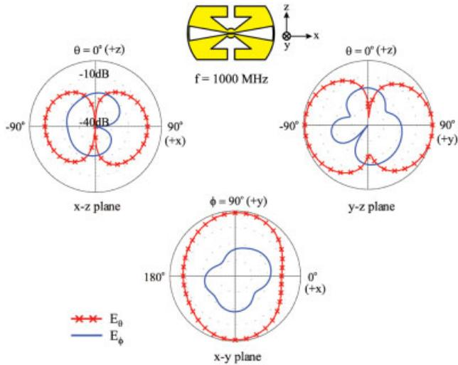
**Figure 7** Measured radiation pattern at 1000 MHz for the proposed antenna studied in Figure 3. [Color figure can be viewed in the online issue, which is available at [www.interscience.wiley.com](http://www.interscience.wiley.com)]
