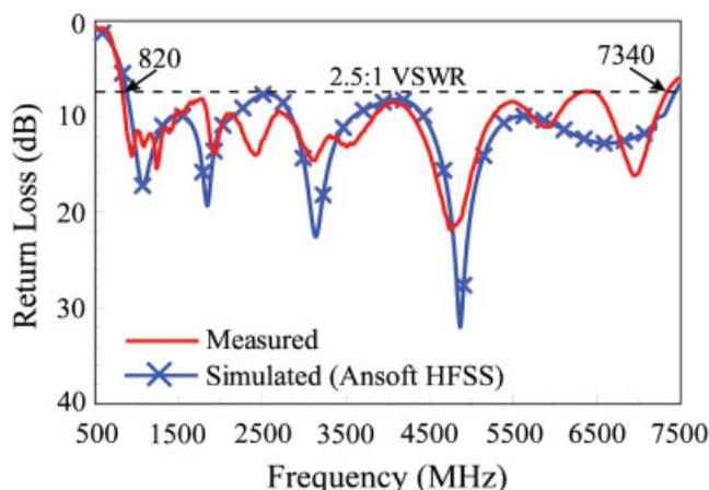
**Figure 3** Measured and simulated return loss for the proposed antenna with preferred dimensions given in Figure 1. [Color figure can be viewed in the online issue, which is available at www.interscience.wiley.com]
