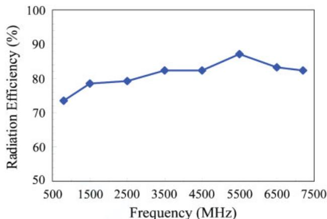
**Figure 11** Simulated radiation efficiency for the proposed antenna studied in Figure 3. [Color figure can be viewed in the online issue, which is available at [www.interscience.wiley.com](http://www.interscience.wiley.com)]
