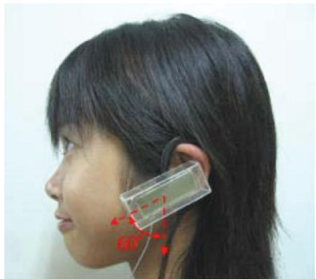
**Figure 7** Photo of the constructed Bluetooth headset antenna attached to a user's head in the experiment. [Color figure can be viewed in the online issue, which is available at [www.interscience.wiley.com](http://www.interscience.wiley.com)]
