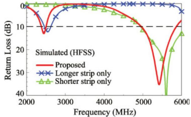
**Figure 4** Simulated return loss for the proposed antenna, the case with the longer strip only, and the case with the shorter strip only. [Color figure can be viewed in the online issue, which is available at [www.interscience.wiley.com](http://www.interscience.wiley.com)]
