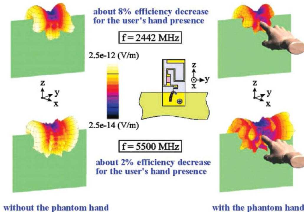
**Figure 10** Simulated 3D radiation patterns at 2442 MHz and 5500 MHz for the proposed antenna with and without the phantom hand. [Color figure can be viewed in the online issue, which is available at [www.interscience.wiley.com](http://www.interscience.wiley.com)]
