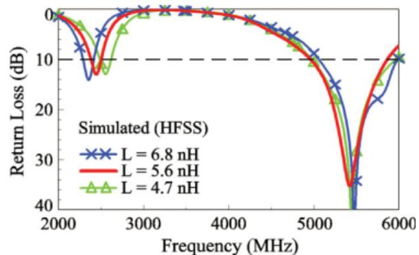
**Figure 5** Simulated return loss of the proposed antenna as a function of the inductance  $L$  of the embedded chip inductor. [Color figure can be viewed in the online issue, which is available at [www.interscience.wiley.com](http://www.interscience.wiley.com)]
