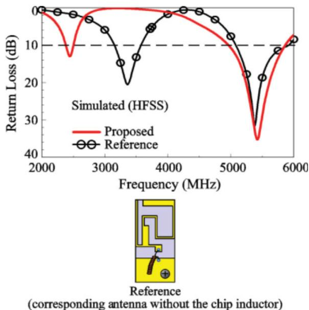
**Figure 3** Simulated return loss for the proposed antenna and the reference antenna (the corresponding design without the chip inductor). [Color figure can be viewed in the online issue, which is available at [www.interscience.wiley.com](http://www.interscience.wiley.com)]
