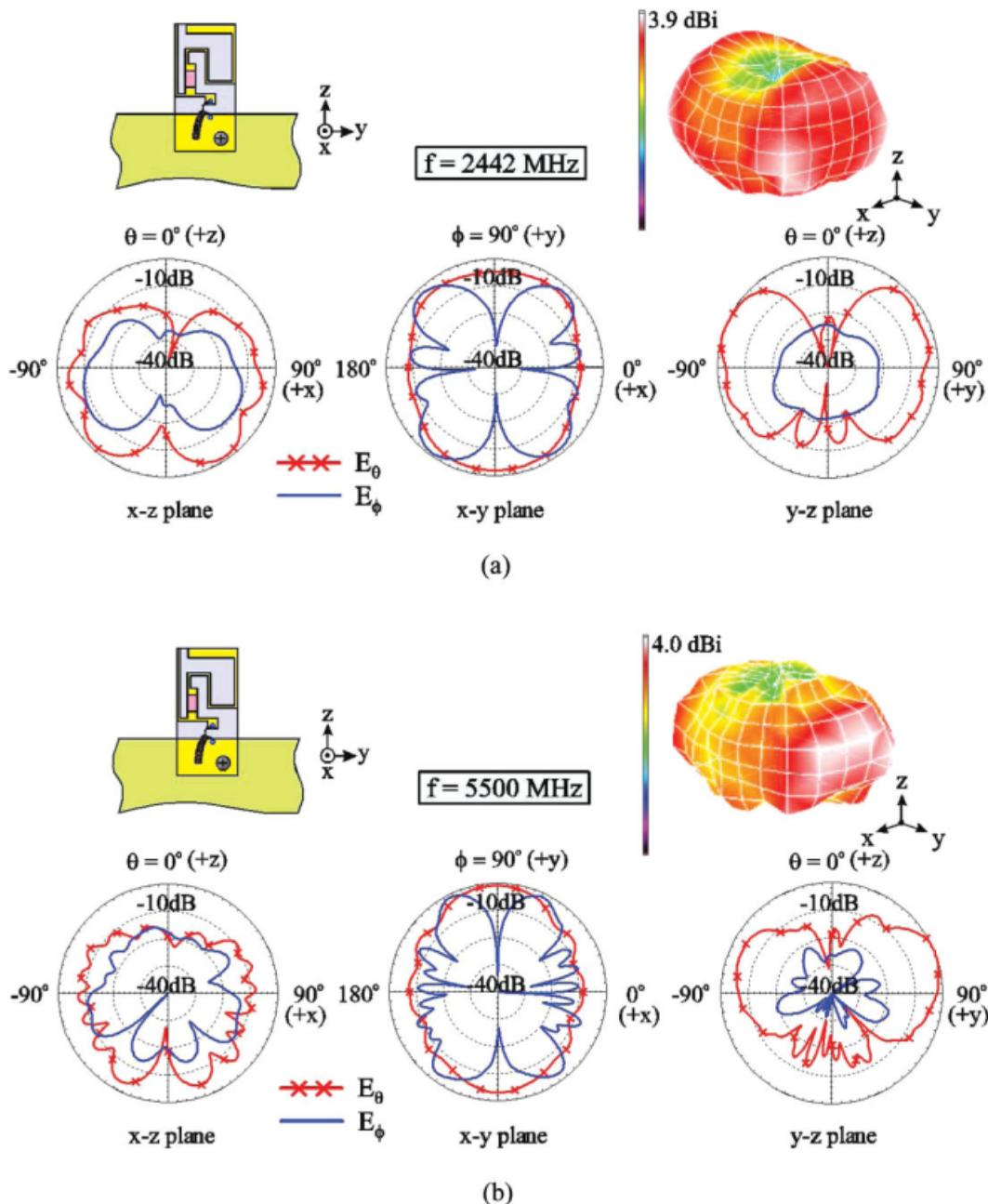
**Figure 6** Measured 2D and 3D radiation patterns at (a) 2442 MHz and (b) 5500 MHz for the proposed antenna. [Color figure can be viewed in the online issue, which is available at [www.interscience.wiley.com](http://www.interscience.wiley.com)]
