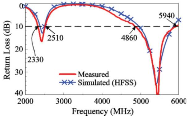
**Figure 2** Measured and simulated return loss for the proposed antenna. [Color figure can be viewed in the online issue, which is available at [www.interscience.wiley.com](http://www.interscience.wiley.com)]
