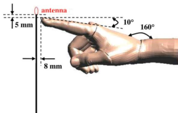
**Figure 8** Simulation model for the proposed antenna with the phantom hand provided by SEMCAD-X [22]. [Color figure can be viewed in the online issue, which is available at [www.interscience.wiley.com](http://www.interscience.wiley.com)]
