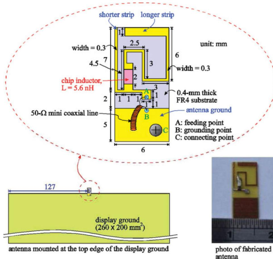
**Figure 1** Geometry of the proposed printed monopole antenna embedded with a chip inductor for 2.4/5.2/5.8 GHz triple-band WLAN operation in the laptop computer. [Color figure can be viewed in the online issue, which is available at [www.interscience.wiley.com](http://www.interscience.wiley.com)]
