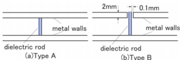
**Figure 5** (a) Dielectric rod located in a waveguide without gaps at top and bottom. (b) Dielectric rod inserted in a hole made at the top of the waveguide with a diameter 0.2 mm larger than the diameter of the rod. [Color figure can be viewed in the online issue, which is available at [www.interscience.wiley.com](http://www.interscience.wiley.com)]
