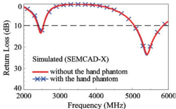
**Figure 9** Simulated return loss for the proposed antenna with and without the phantom hand. [Color figure can be viewed in the online issue, which is available at [www.interscience.wiley.com](http://www.interscience.wiley.com)]
