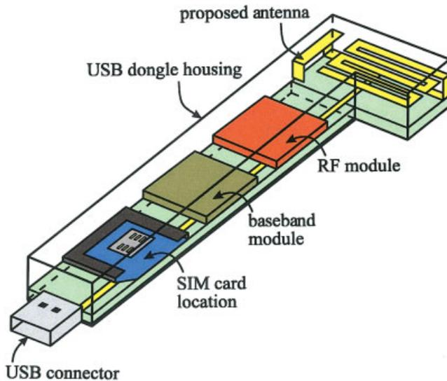
**Figure 2** Example of a promising USB dongle with the proposed antenna. [Color figure can be viewed in the online issue, which is available at [www.interscience.wiley.com](http://www.interscience.wiley.com)]
