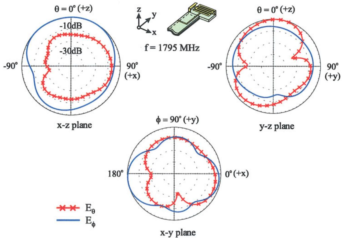
**Figure 6** Measured radiation patterns at 1795 MHz for the antenna shown in Figure 1. [Color figure can be viewed in the online issue, which is available at [www.interscience.wiley.com](http://www.interscience.wiley.com)]
