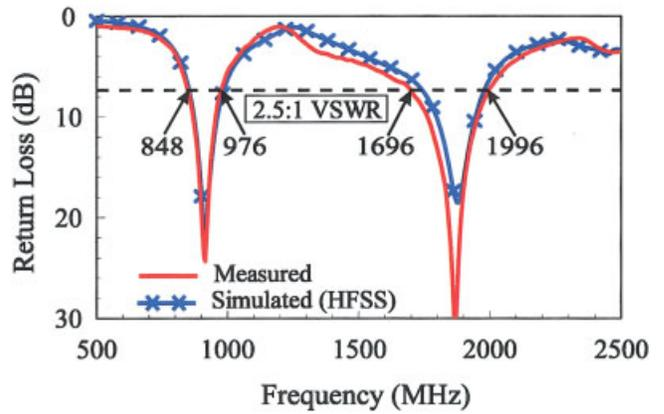
**Figure 3** Measured and simulated return loss of the proposed antenna. [Color figure can be viewed in the online issue, which is available at [www.interscience.wiley.com](http://www.interscience.wiley.com)]
