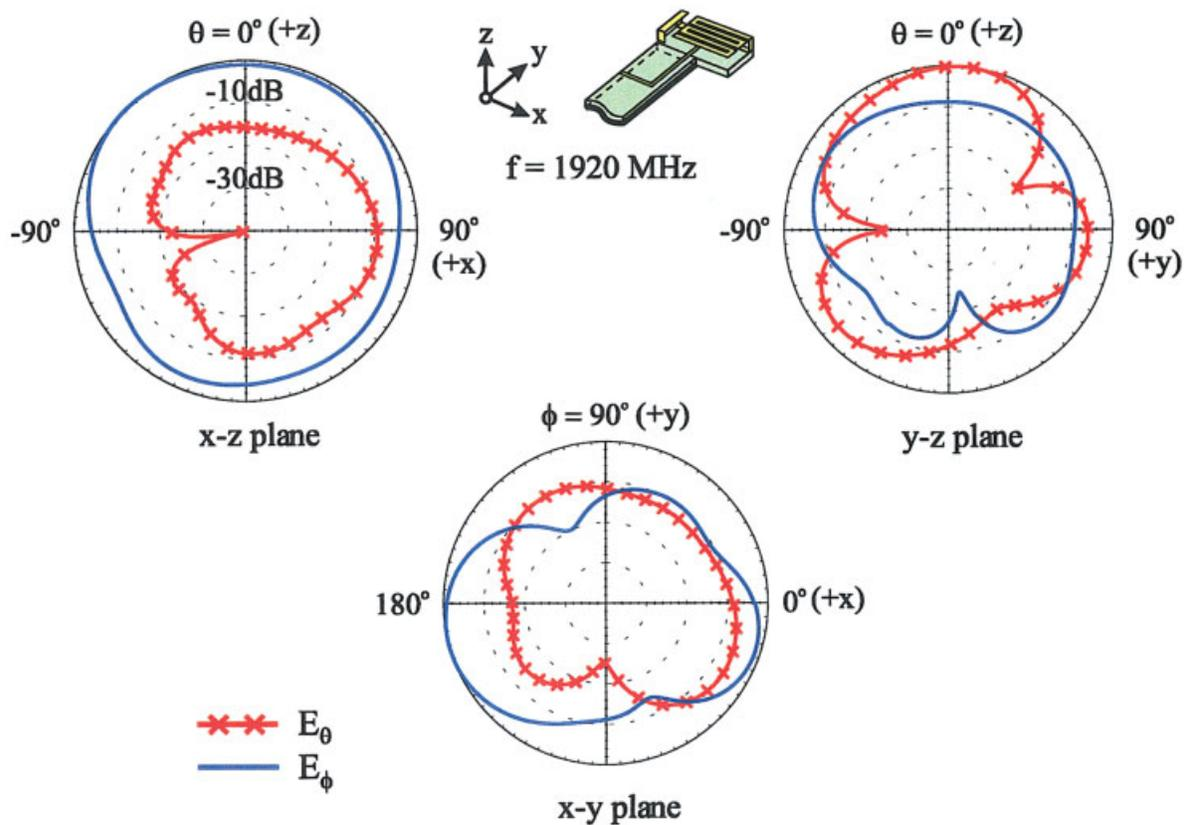
**Figure 7** Measured radiation patterns at 1920 MHz for the antenna shown in Figure 1. [Color figure can be viewed in the online issue, which is available at [www.interscience.wiley.com](http://www.interscience.wiley.com)]
