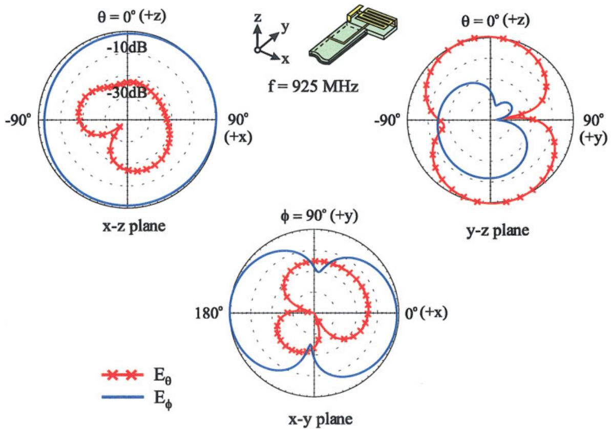
**Figure 5** Measured radiation patterns at 925 MHz for the antenna shown in Figure 1. [Color figure can be viewed in the online issue, which is available at [www.interscience.wiley.com](http://www.interscience.wiley.com)]
