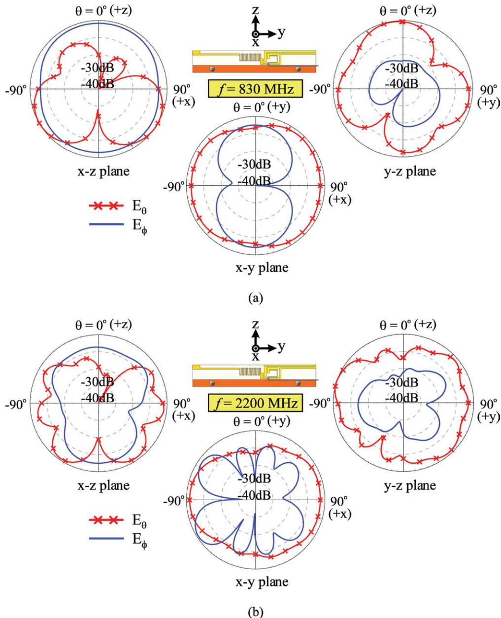
**Figure 6** Measured radiation patterns at (a) 830 MHz and (b) 2200 MHz for the proposed antenna. [Color figure can be viewed in the online issue, which is available at [www.interscience.wiley.com](http://www.interscience.wiley.com)]
