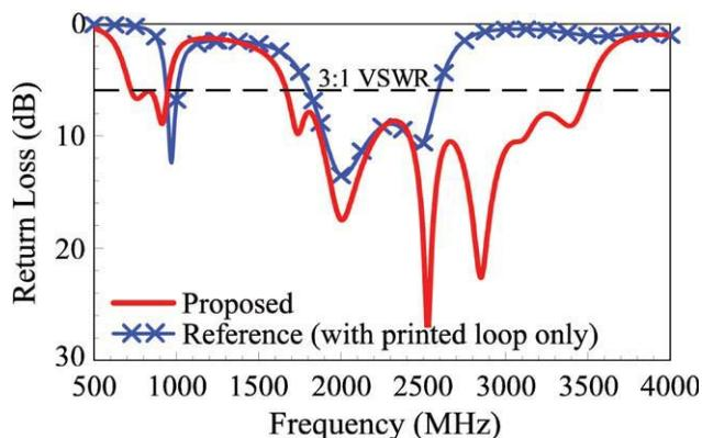
**Figure 3** Simulated return loss for the proposed antenna and the case with the printed loop only. [Color figure can be viewed in the online issue, which is available at [www.interscience.wiley.com](http://www.interscience.wiley.com)]
