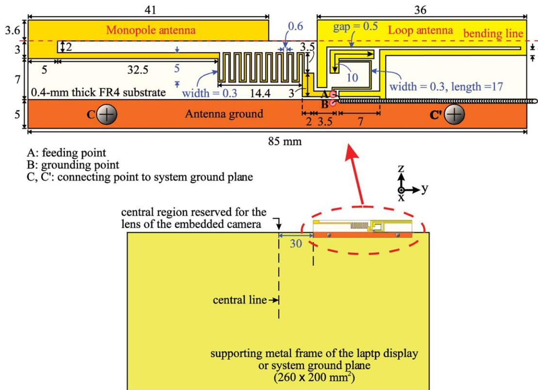
**Figure 1** Geometry of the proposed printed loop/monopole combo antenna mounted along the top edge of the supporting metal frame of the display panel in the laptop computer for LTE/GSM/UMTS operation. [Color figure can be viewed in the online issue, which is available at [www.interscience.wiley.com](http://www.interscience.wiley.com)]
