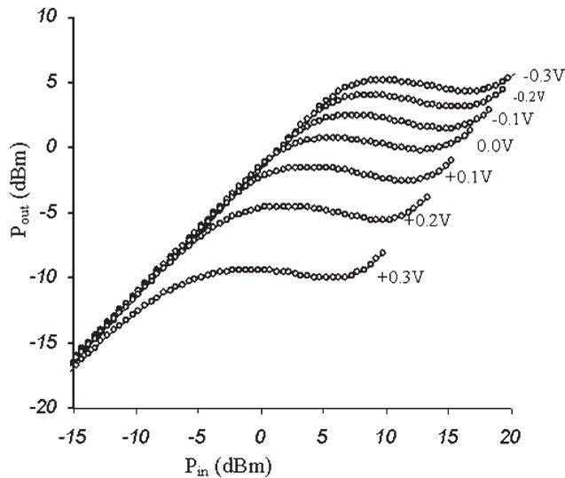
**Figure 6** Tested  $P_{in}$  Vs  $P_{out}$  of the limiter at different control voltages
