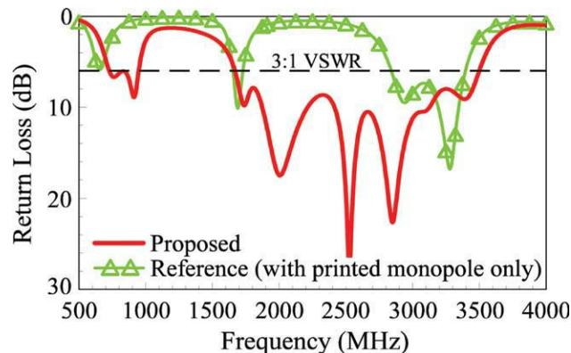
**Figure 4** Simulated return loss for the proposed antenna and the case with the printed monopole only. [Color figure can be viewed in the online issue, which is available at [www.interscience.wiley.com](http://www.interscience.wiley.com)]
