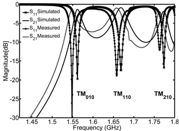
Figure 5 Magnitude of measured and simulated S-parameters
