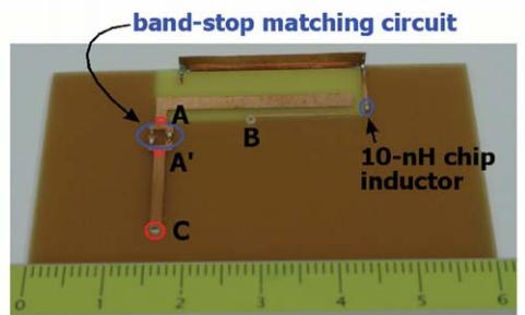
A'C: 50-Ω feedline for testing the antenna
