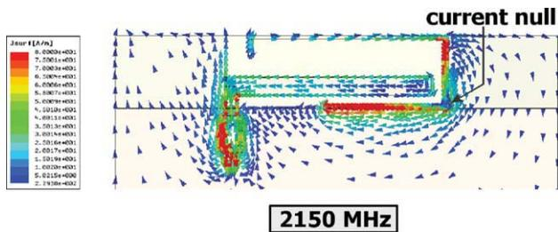
**Figure 4** Simulated surface current distributions at 2150 MHz for the proposed antenna. [Color figure can be viewed in the online issue, which is available at [wileyonlinelibrary.com](http://wileyonlinelibrary.com)]
