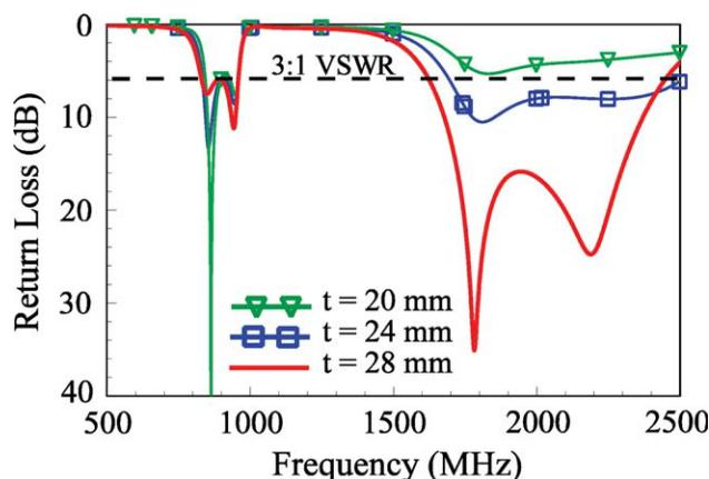
**Figure 7** Simulated return loss as a function of the length  $t$  in the driven strip monopole for the proposed antenna. [Color figure can be viewed in the online issue, which is available at [wileyonlinelibrary.com](http://wileyonlinelibrary.com)]
