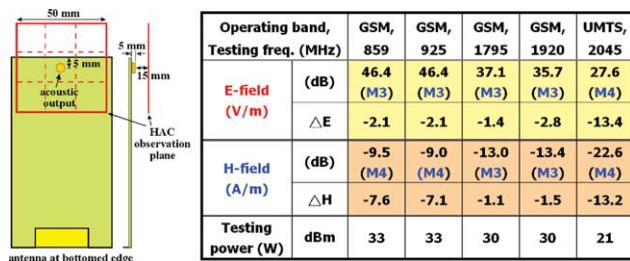
**Figure 11** HAC simulation model and the simulated HAC results.  $\Delta E$  and  $\Delta H$  indicate, respectively, the decrease in the E-field and H-field strengths owing to the presence of the two protruded grounds at two side edges of the antenna. [Color figure can be viewed in the online issue, which is available at [wileyonlinelibrary.com](http://wileyonlinelibrary.com)]
