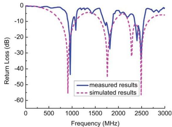
**Figure 8** The measured and simulated values of return loss  $S_{11}$ . [Color figure can be viewed in the online issue, which is available at [wileyonlinelibrary.com](http://wileyonlinelibrary.com)]
