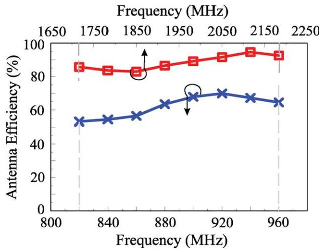
**Figure 8** Measured antenna efficiency (mismatching loss included) of the proposed antenna. [Color figure can be viewed in the online issue, which is available at [wileyonlinelibrary.com](http://wileyonlinelibrary.com)]
