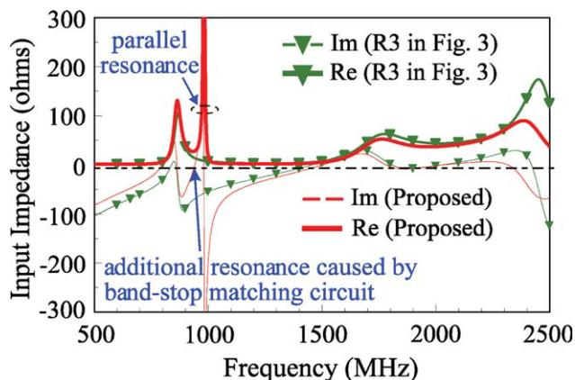
**Figure 5** Simulated return loss for the proposed antenna and the case without the band-stop matching circuit (R3 in Fig. 3). [Color figure can be viewed in the online issue, which is available at [wileyonlinelibrary.com](http://wileyonlinelibrary.com)]
