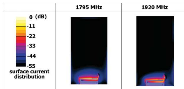
**Figure 12** Simulated surface current distributions on the system ground plane. [Color figure can be viewed in the online issue, which is available at [wileyonlinelibrary.com](http://wileyonlinelibrary.com)]
