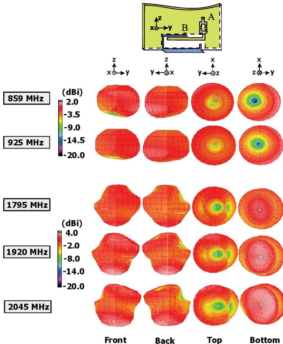
**Figure 9** Measured three-dimensional total-power radiation patterns of the proposed antenna. [Color figure can be viewed in the online issue, which is available at [wileyonlinelibrary.com](http://wileyonlinelibrary.com)]
