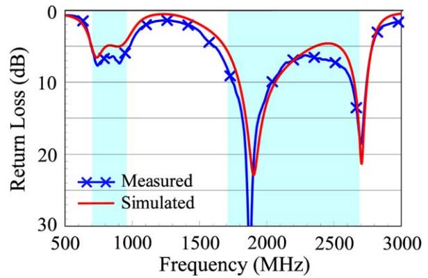
**Figure 5** Measured and simulated return loss of the fabricated antenna. [Color figure can be viewed in the online issue, which is available at [wileyonlinelibrary.com](http://wileyonlinelibrary.com)]
