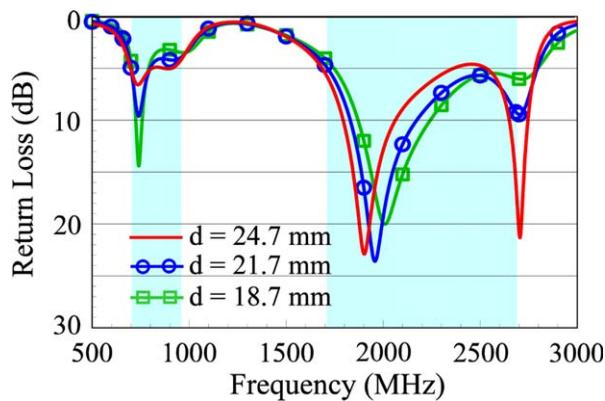
**Figure 10** Simulated return loss as a function of the length  $d$  in the feeding strip. Other dimensions are the same as in Figure 1. [Color figure can be viewed in the online issue, which is available at wileyonlinelibrary.com]
