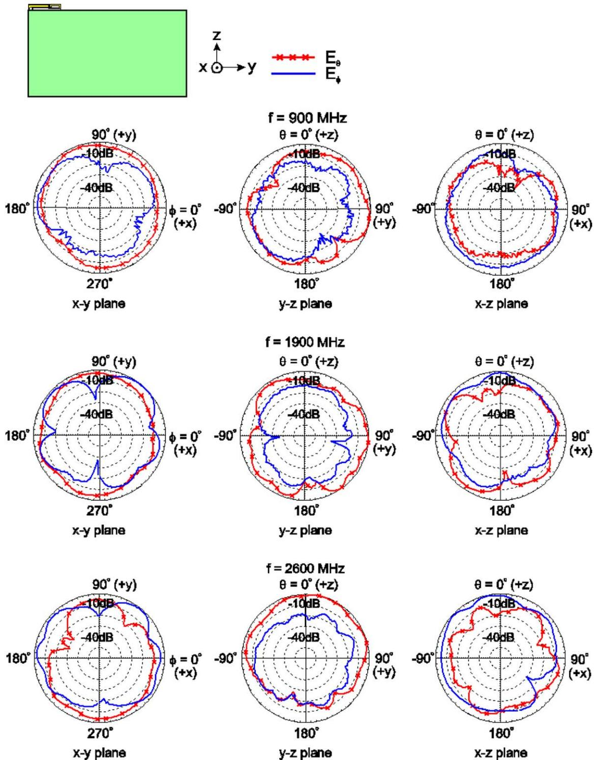
**Figure 7** Measured radiation patterns at 900, 1900, and 2600 MHz of the fabricated antenna. [Color figure can be viewed in the online issue, which is available at [wileyonlinelibrary.com](http://wileyonlinelibrary.com)]
