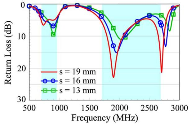
**Figure 11** Simulated return loss as a function of the length  $s$  in the shorted folded strip. Other dimensions are the same as in Figure 1.
