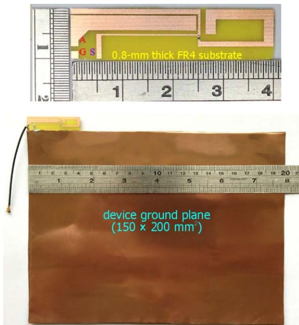
**Figure 4** Photos of the fabricated antenna and the same with the device ground plane for experimental testing. [Color figure can be viewed in the online issue, which is available at [wileyonlinelibrary.com](http://wileyonlinelibrary.com)]
