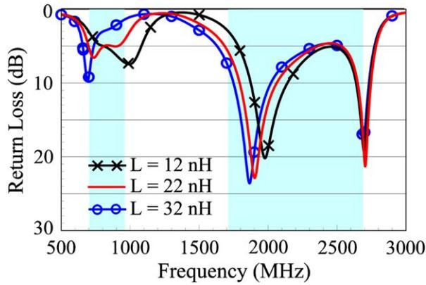
**Figure 8** Simulated return loss as a function of the inductance  $L$  of the chip inductor. Other dimensions are the same as in Figure 1. [Color figure can be viewed in the online issue, which is available at wileyonlinelibrary.com]
