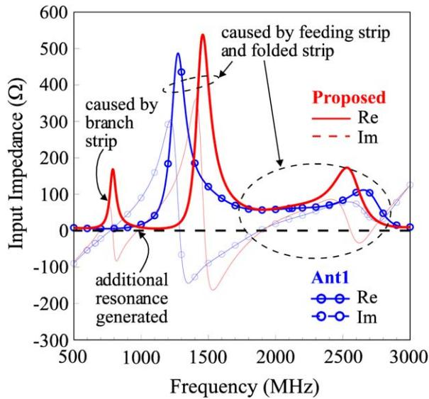
**Figure 3** Simulated input impedance for the proposed antenna shown in Figure 1 and Ant1 shown in Figure 2. [Color figure can be viewed in the online issue, which is available at [wileyonlinelibrary.com](http://wileyonlinelibrary.com)]
