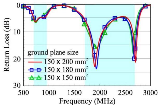
**Figure 12** Simulated return loss as a function of the device ground plane size. [Color figure can be viewed in the online issue, which is available at wileyonlinelibrary.com]
