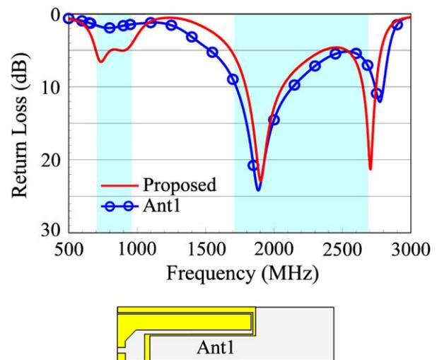
**Figure 2** Simulated return loss for the proposed antenna and the case with the coupled-fed shorted strip antenna only (Ant1, no branch strip). Corresponding dimensions are the same as given in Figure 1. [Color figure can be viewed in the online issue, which is available at [wileyonlinelibrary.com](http://wileyonlinelibrary.com)]
