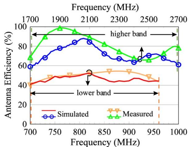
**Figure 6** Measured antenna efficiency of the fabricated antenna. [Color figure can be viewed in the online issue, which is available at [wileyonlinelibrary.com](http://wileyonlinelibrary.com)]
