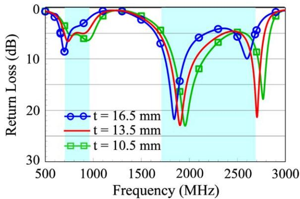
**Figure 9** Simulated return loss as a function of the length  $t$  in the branch strip. [Color figure can be viewed in the online issue, which is available at wileyonlinelibrary.com]
