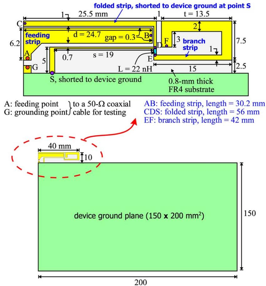
**Figure 1** Geometry of the proposed LTE/WWAN tablet computer antenna. [Color figure can be viewed in the online issue, which is available at [wileyonlinelibrary.com](http://wileyonlinelibrary.com)]
