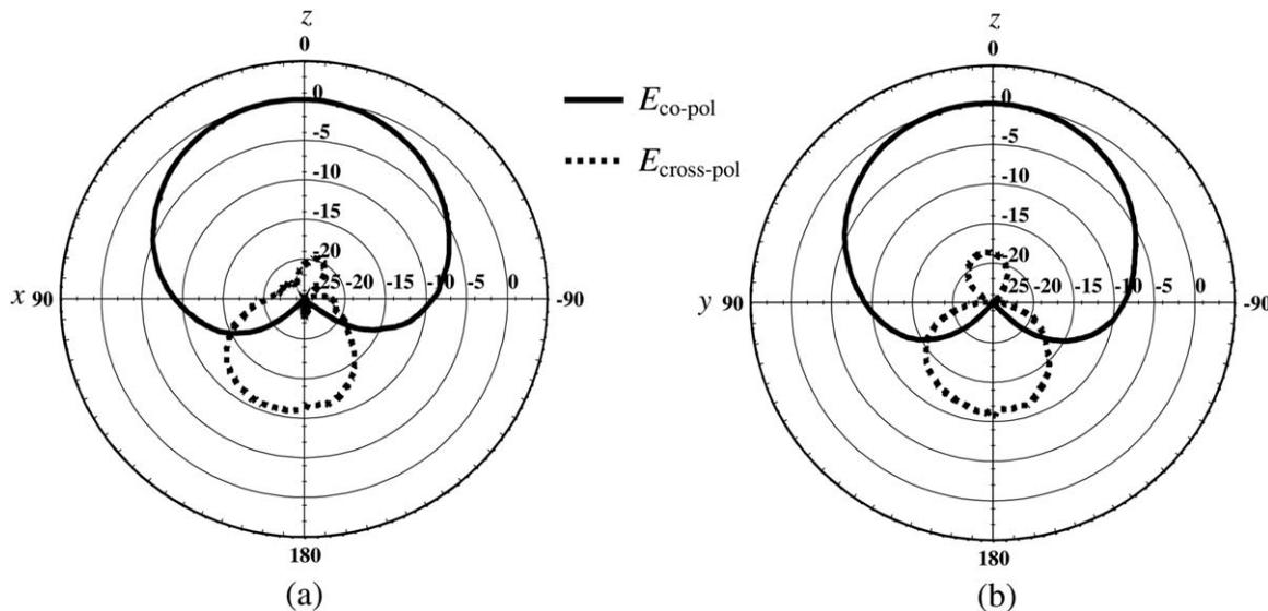
**Figure 8** Measured radiation patterns at 1.575 GHz for the prototype with  $C = 0.9$  pF. (a)  $x$ - $z$  plane and (b)  $y$ - $z$  plane
