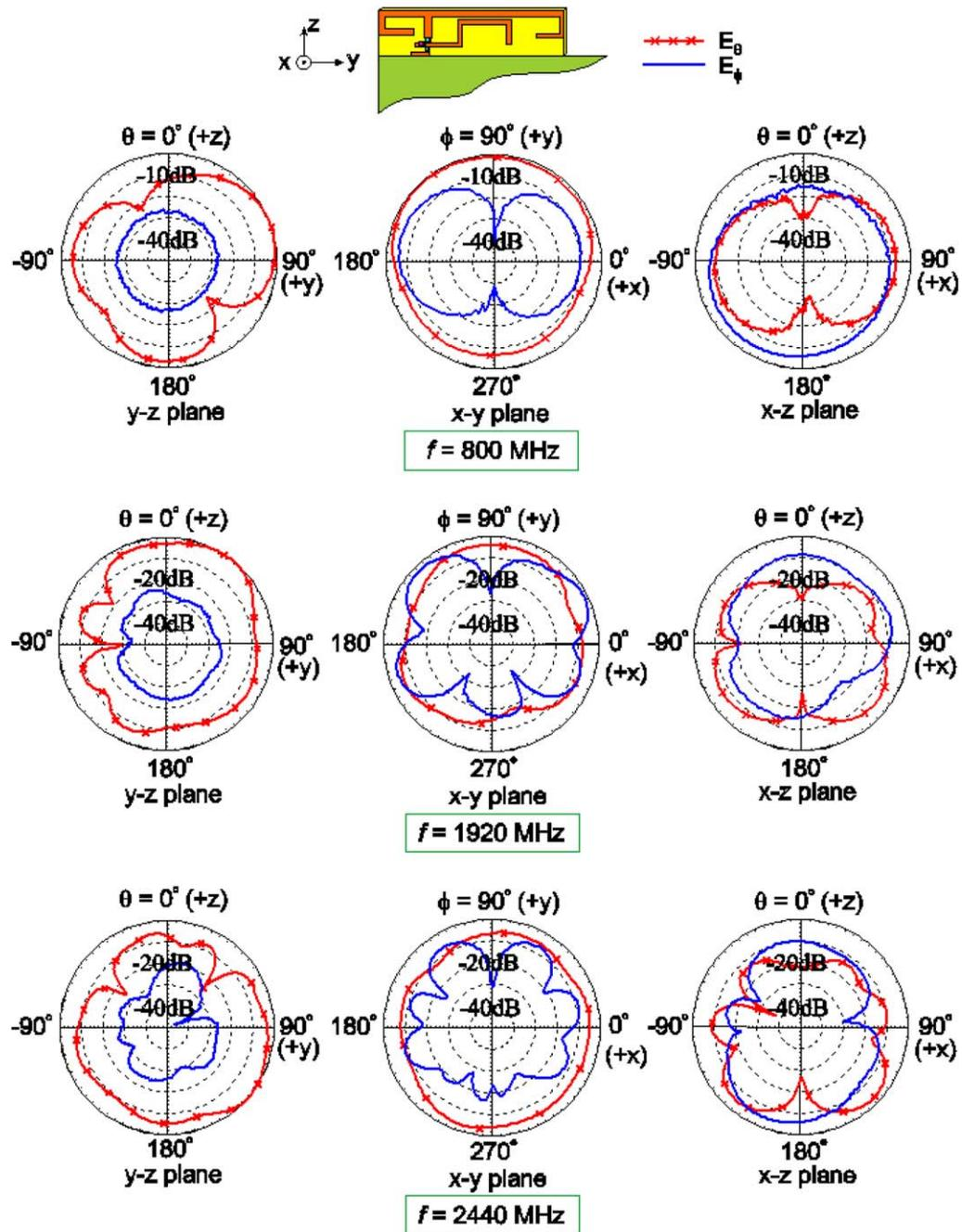
**Figure 9** Measured radiation patterns of the fabricated antenna. [Color figure can be viewed in the online issue, which is available at [wileyonlinelibrary.com](http://wileyonlinelibrary.com)]
