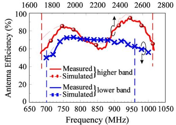
**Figure 8** Measured and simulated antenna efficiency (matching loss included) of the fabricated antenna. [Color figure can be viewed in the online issue, which is available at [wileyonlinelibrary.com](http://wileyonlinelibrary.com)]
