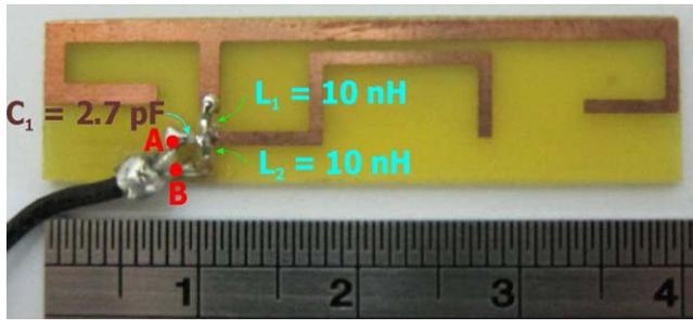
**Figure 2** Photo of the fabricated antenna. [Color figure can be viewed in the online issue, which is available at [wileyonlinelibrary.com](http://wileyonlinelibrary.com)]
