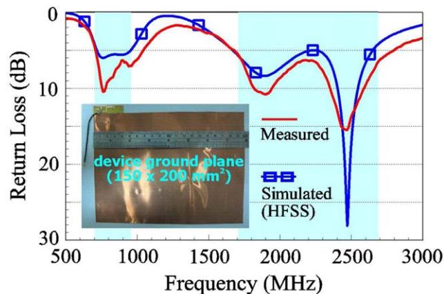
**Figure 7** Measured and simulated return loss of the fabricated antenna. [Color figure can be viewed in the online issue, which is available at [wileyonlinelibrary.com](http://wileyonlinelibrary.com)]
