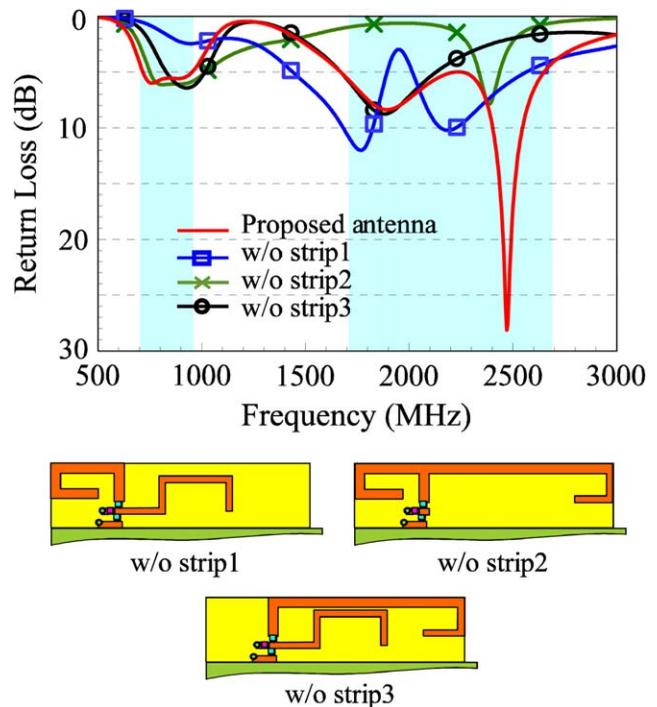
**Figure 5** Simulated return loss for the proposed antenna, the case without Strip1, the case without Strip2, and the case without Strip3. [Color figure can be viewed in the online issue, which is available at [wileyonlinelibrary.com](http://wileyonlinelibrary.com)]
