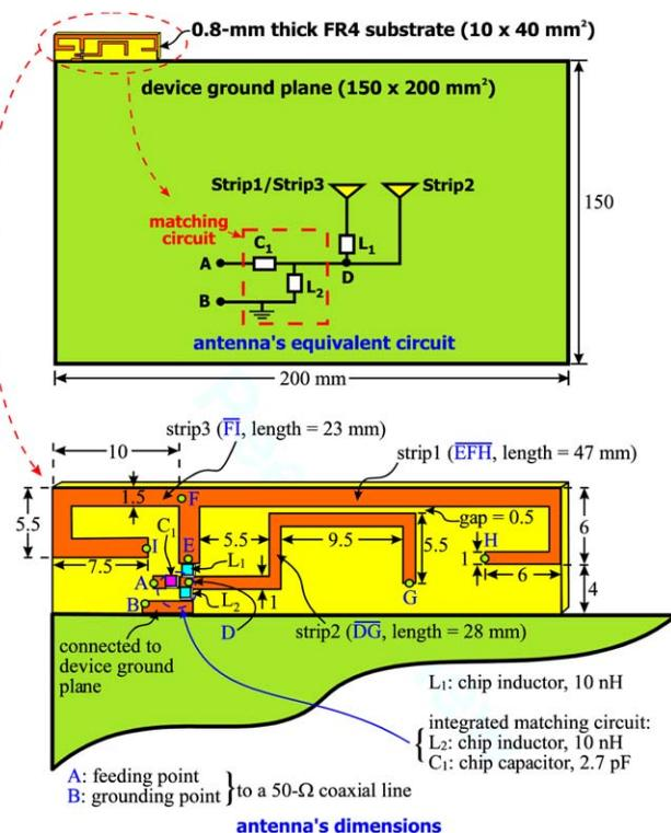
**Figure 1** Geometry of the proposed LTE/WWAN/WLAN tablet computer antenna. [Color figure can be viewed in the online issue, which is available at [wileyonlinelibrary.com](http://wileyonlinelibrary.com)]
