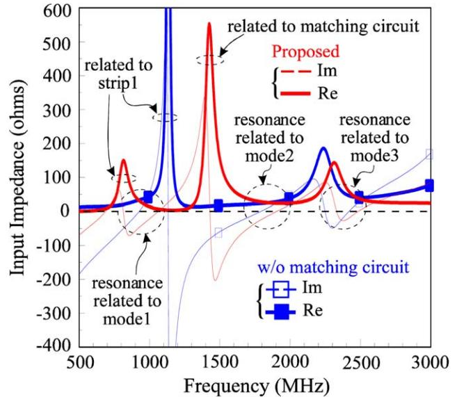
**Figure 4** Simulated input impedance for the proposed antenna and the case without the integrated matching circuit. [Color figure can be viewed in the online issue, which is available at [wileyonlinelibrary.com](http://wileyonlinelibrary.com)]
