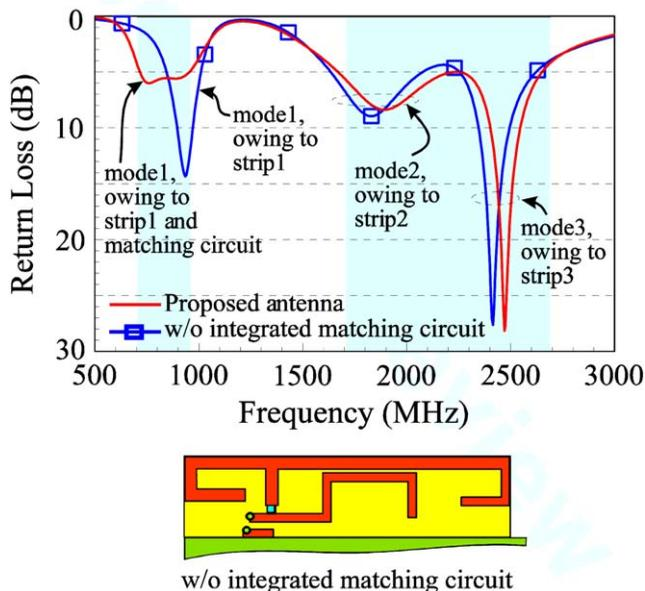
**Figure 3** Simulated return loss for the proposed antenna and the case without the integrated matching circuit. [Color figure can be viewed in the online issue, which is available at [wileyonlinelibrary.com](http://wileyonlinelibrary.com)]
