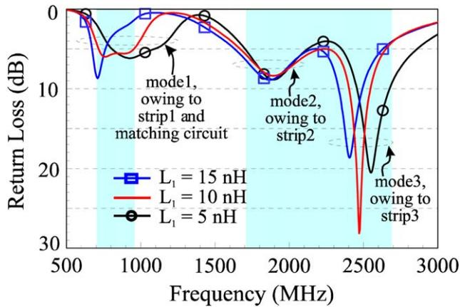
**Figure 6** Simulated return loss as a function of the chip inductor  $L_1$ . [Color figure can be viewed in the online issue, which is available at [wileyonlinelibrary.com](http://wileyonlinelibrary.com)]
