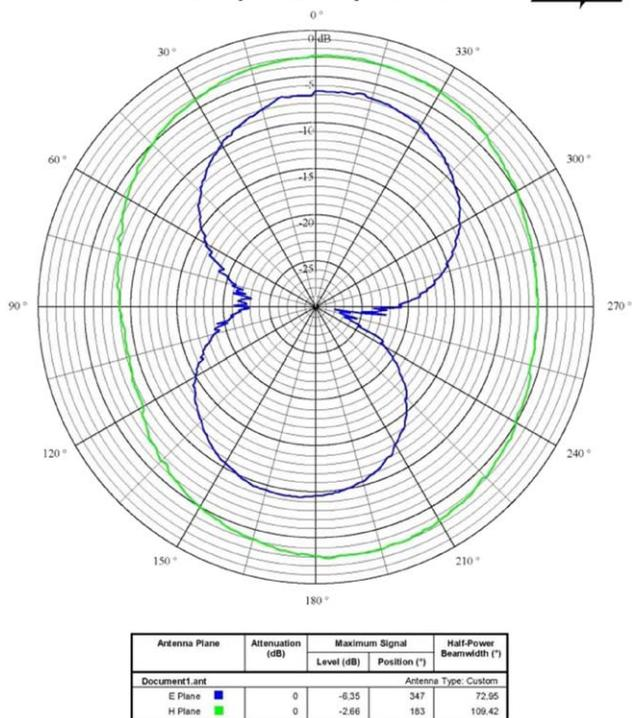
**Figure 11** The measured radiation using Labvolt for the setup with the superstrate. [Color figure can be viewed in the online issue, which is available at [wileyonlinelibrary.com](http://wileyonlinelibrary.com)]
