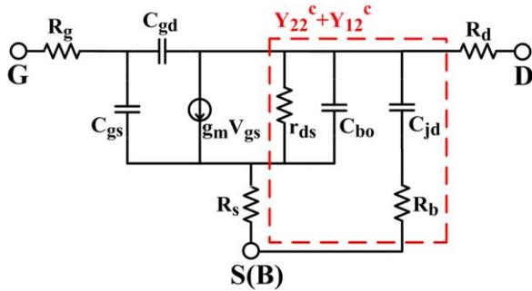
**Figure 7** A small-signal equivalent circuit model of a RF SOI MOSFET under CSB configuration. [Color figure can be viewed at wileyonlinelibrary.com]
